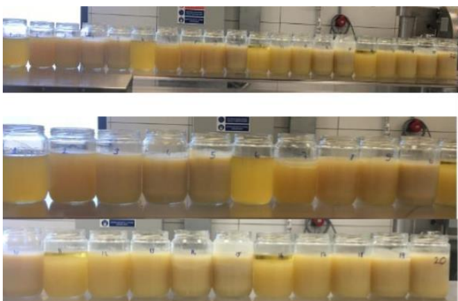
Figure 1. The samples prepared with different types of waxes and lecithins according to experimental design.
