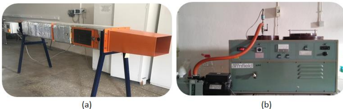
Fig. 2 Pilot-scale hot air dryer (a), pilot-scale freeze dryer (b)
